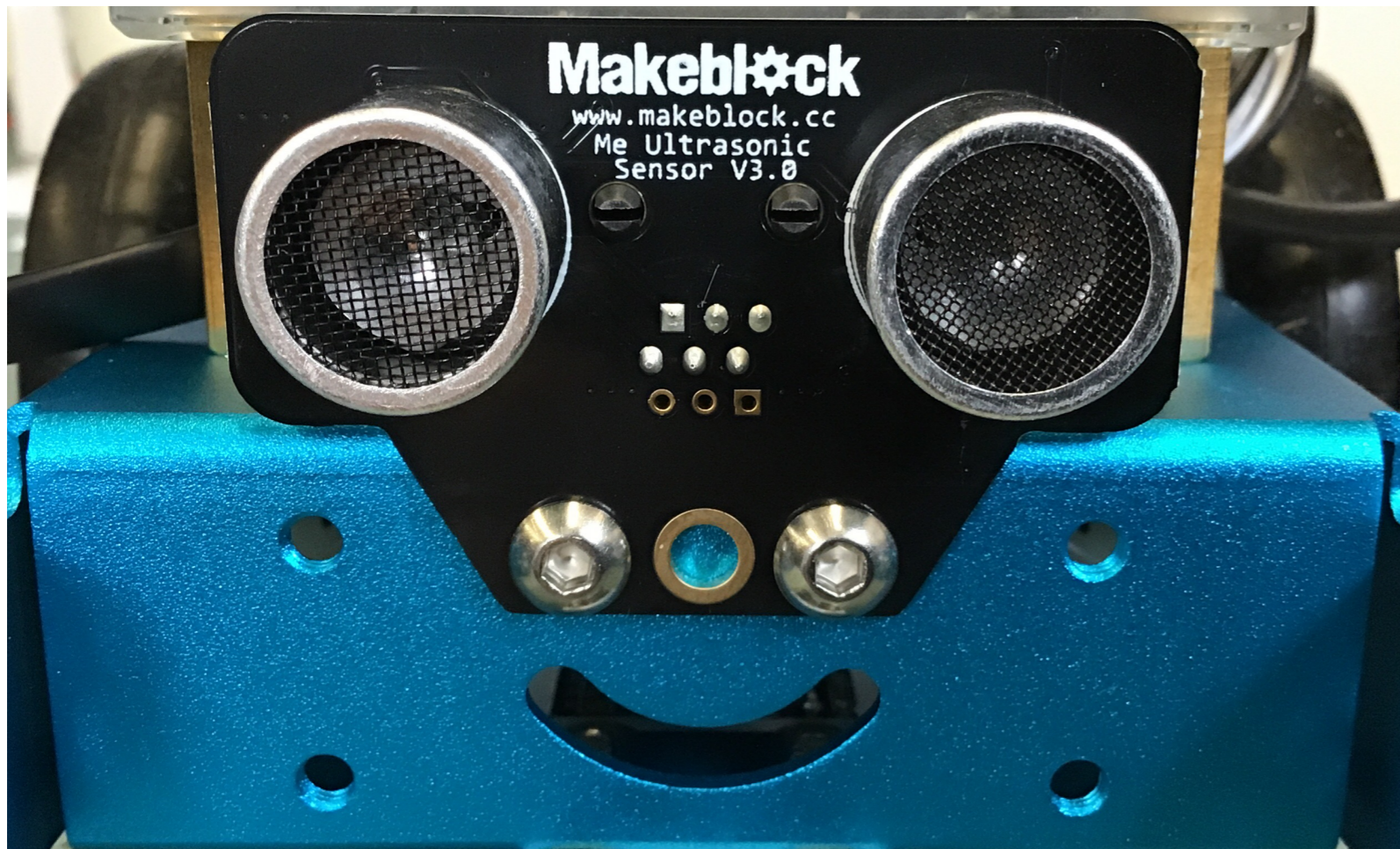
A closeup of the mBot's "face". The eyes are the Ultrasonic sensor.
